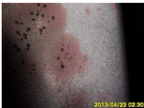
Figure 4. The impact of droplets on the surface of the 22 stage blades of medium-pressure rotor
