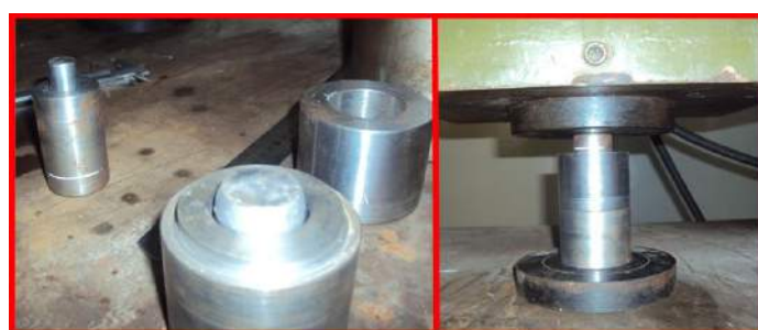
Figure 7. Preparing the work piece inside the die and the process of pressing
